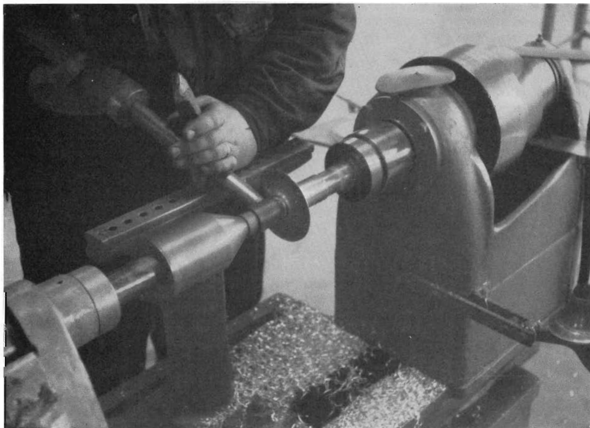
Metal spinning operation in country factory established with Commission assistance.
