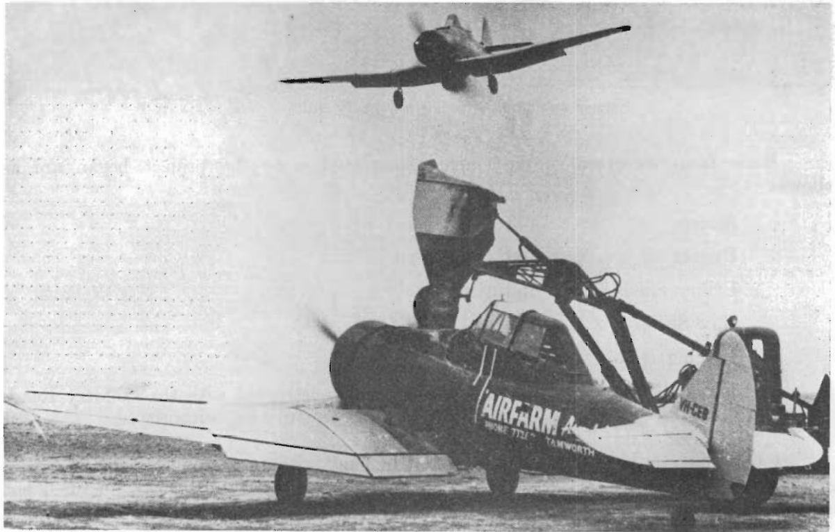
Loading of aircraft with superphosphate for spreading on pastures at Heytesbury settlement area.
