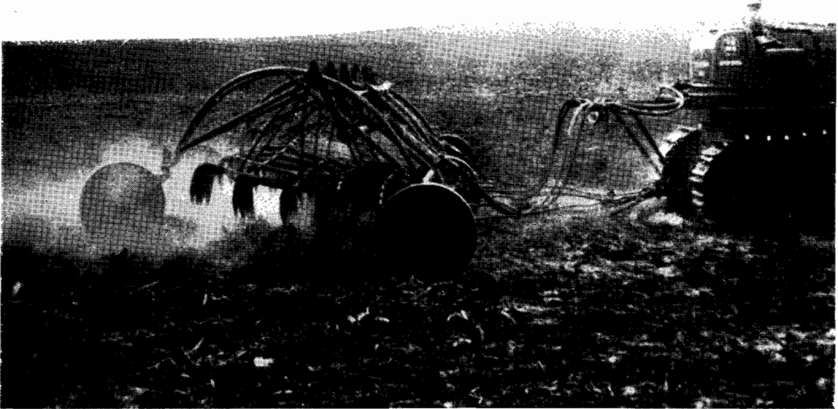
Special Harrows Developed by the Commission for Handling Debris in the Development of Crown Lands.
