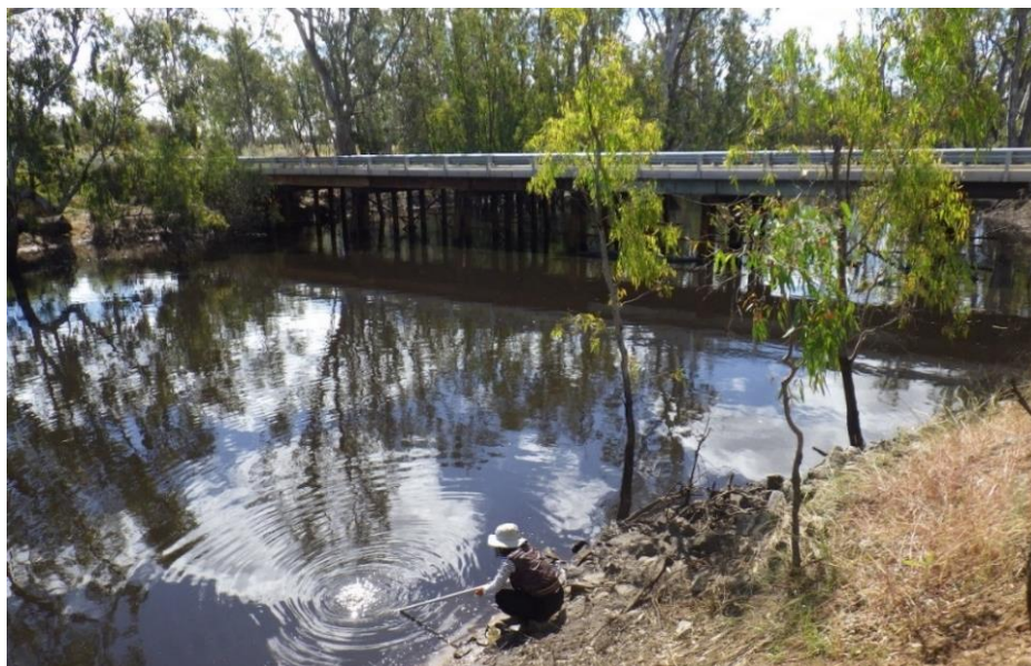
Photo 2: Collecting water quality samples from Thule Creek which runs through the Koondrook Forest. The dark water colour indicates high dissolved organic carbon (around 25 mg/L on this date) and the dissolved oxygen was low (1.9 mg/L). (Photo: Nicole McCasker 14/11/2016)
