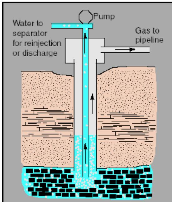
Figure 1: Coal Seam Gas Extraction (Source: DPI)
