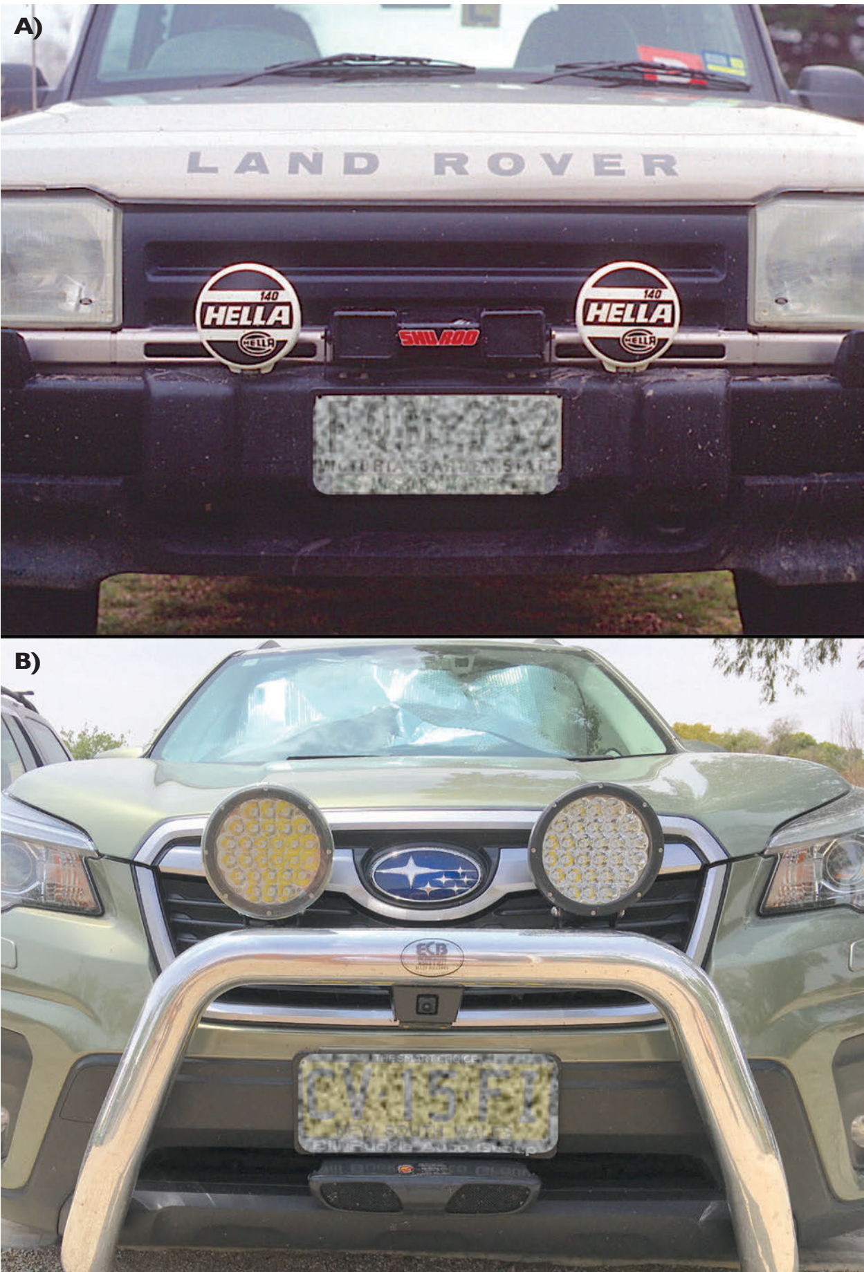
Figure 1. Vehicles fitted with the ShuRoo: (a) Mark 1, (b) Mark 5. Note the powerful driving lights also fitted to both vehicles.
