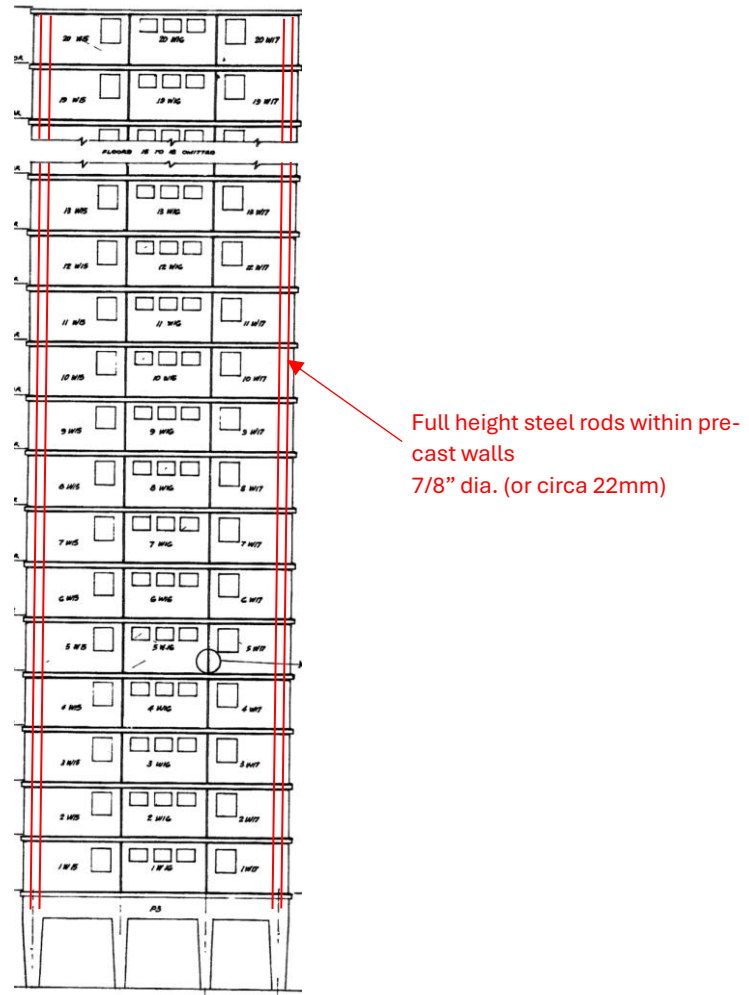
Figure 13 – Elevation view of westernmost wall of west wing indicating full height tension rods within wall panels.
