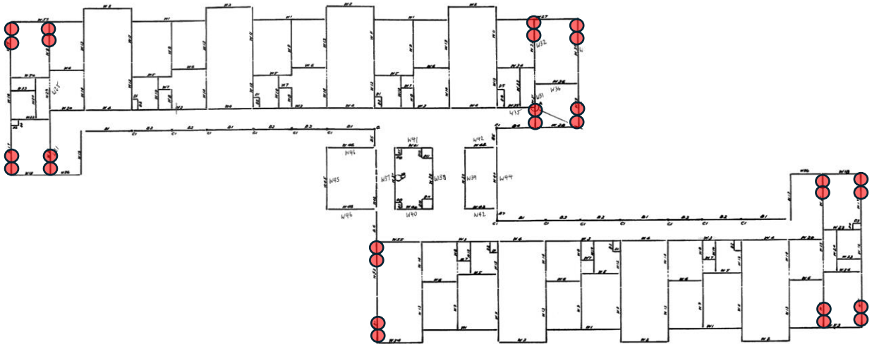
Figure 12 – Plan view of typical floor identifying location of full building height tension rods embedded within wall panels (not to scale)
