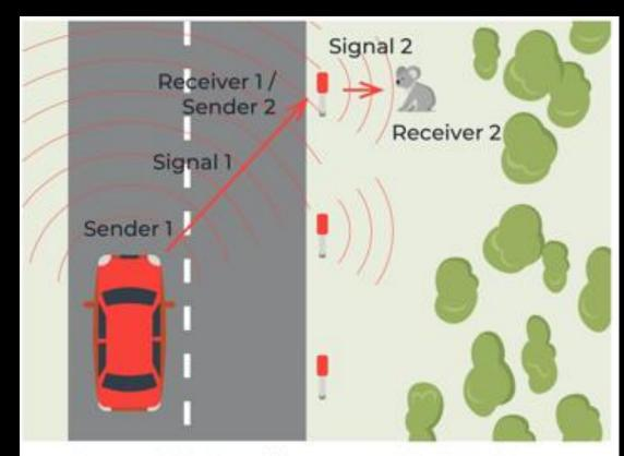
Sender 1: Vehicle | Receiver 1: Wayside detection system Sender 2: Wayside deterrent system | Receiver 2: Wildlife
