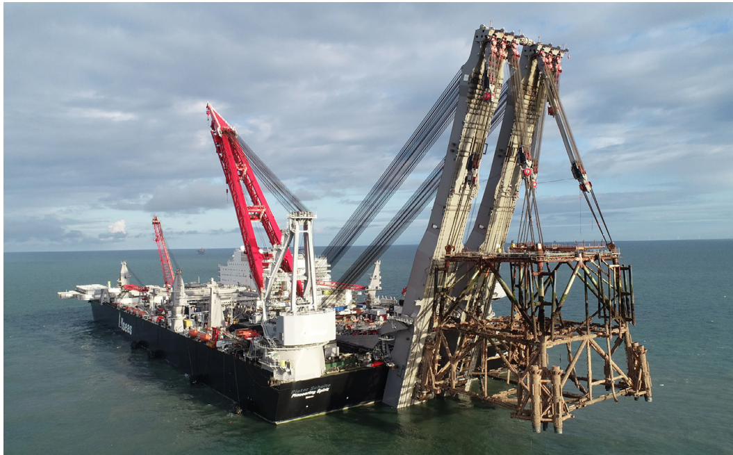
Figure 2.7 Allseas Pioneering Spirit removing subsea infrastructure
