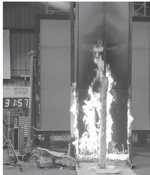
**Image:** This test explored vertical fire spread in a worst-case scenario where a flashover occurs in the unit directly below and fire has entered the wall cavity.
