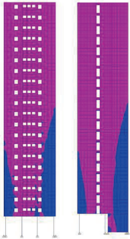
Figure 3. Elevation of the westmost primary load-bearing wall (Left) and the next internal wall immediately to the east (Right). This indicates locations where the walls are overstressed based on seismic loading conditions (blue shaded area). Image by Sheer Force Engineering. Source (OFFICE 2024: p. 61).
