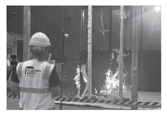
Image: Cladding product fire testing underway.
