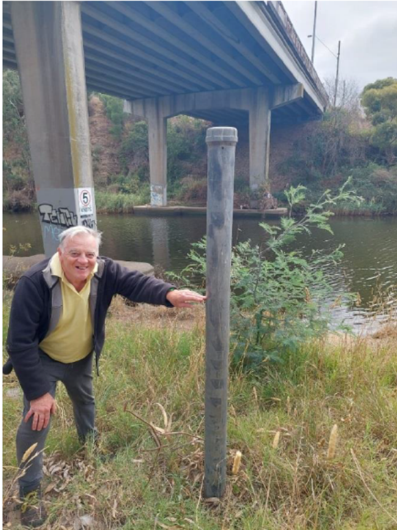
Photo 1 Me pointing to 3.0 m AHD survey datum on old MMBW crest level gauge (left) and Photo 2 sighting the floor level of my flood victim friend's floor level at Rivervue Retirement Village.
